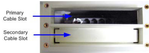
Figure 26: Primary Cable Slot
