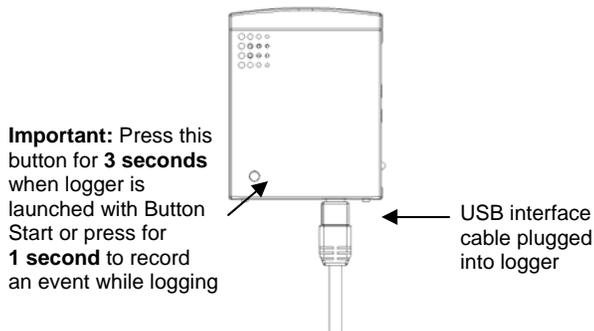
If the logger has never been connected to the computer before, it may take a few seconds for the new hardware to be detected. Use the logger software to launch and read out the logger.
