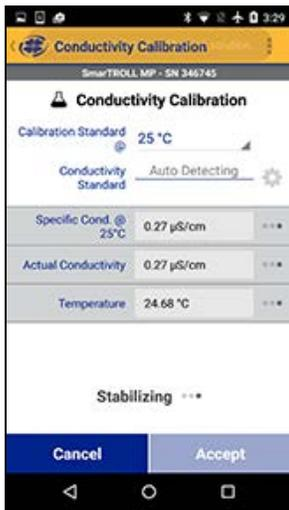
7. Check your bottle of calibration standard to determine the reference temperature. If necessary, tap the drop down list and select the appropriate reference temperature for the calibration.
