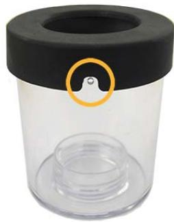
6. Fill the calibration cup to the fill line with calibration standard. Place the instrument in the calibration cup and select **Next**.
