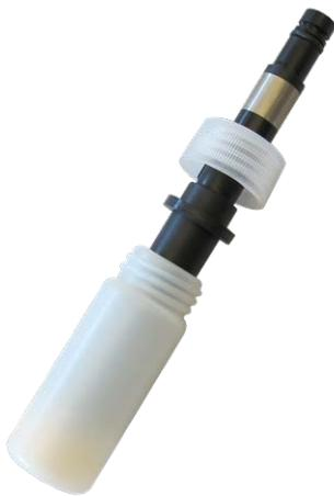
6. Place the sensor tip in the buffer and tighten the cap to prevent the glass bulb from drying.
