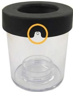
5. Fill the calibration cup to the fill line with calibration standard. Place the instrument in the calibration cup and select **Next**.
