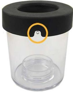
7. Fill the cup to the fill line with Quick-Cal standard. Place the instrument in the calibration cup and select **Next**.
