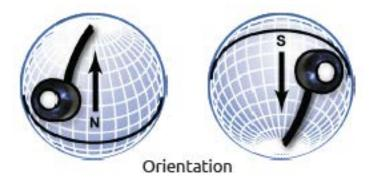
In addition to orienting the cable to point toward the nearest pole, the sensor should also be mounted such that obstructions (e.g., weather station tripod/tower or other instrumentation) do not shade the sensor. **Once mounted, the green cap should be removed from the sensor.** The green cap can be used as a protective covering for the sensor when it is not in use.
