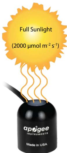
Example of PPFD measurement with an Apogee quantum sensor. Full sunlight yields a PPFD on a horizontal plane at the Earth's surface of approximately  $2000 \mu\text{mol m}^{-2} \text{s}^{-1}$ . This yields an output signal of 4000 mV for the 0-5 V option or an output signal of 2000 mV for the 0-2.5 V option. The signal is converted to PPFD by multiplying by the calibration factor.
