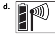
Once the mote has finished joining the network, the "x" icon is removed and the channel count on the station LCD increases by two (one for soil moisture and one for the mote battery).
