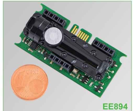
An optional kit for the E2 interface facilitates easy configuration of the module and the adjustment of the CO<sub>2</sub>, RH, T and p measurement. The CO<sub>2</sub> measurement interval can be set according to the application requirements; by this the average current consumption can be reduced to 420 µA, ideal for battery-operated devices.
