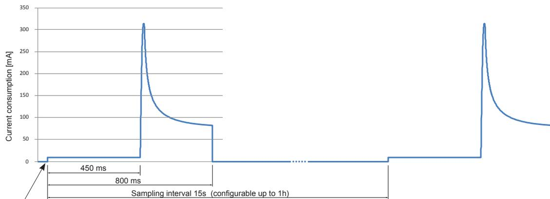
First reading occurs 5...15 seconds after power on, for details see Application Note at [www.epluse.com/ee894](http://www.epluse.com/ee894).
