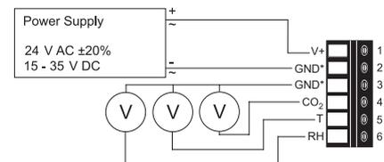
\* **Very important:** for failure-free operation and performance according to the specs the supply GND and the measurement GND must be wired separately.
