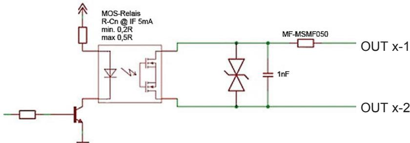
The relay switch and pulse outputs are both potential free.
