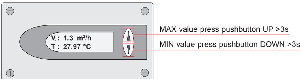
After that the several different measurement values can be indicated using the UP or DOWN keys.
