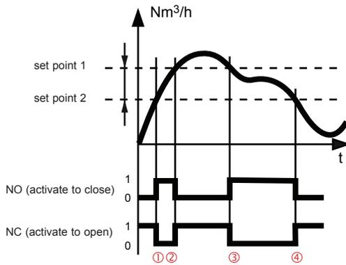
The relay is activated as long as the measuring value is between the values of **set point 1** and **set point 2**. The hysteresis of each set point is fixed at 0.2% of the measuring range.
