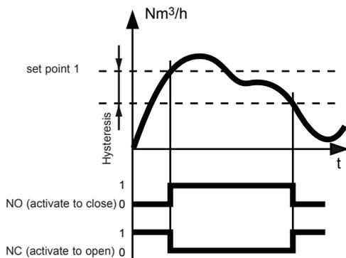
When the measurement value reaches **set point 1**, the relay will be activated. The value at the reset point is the value at set point 1 minus the hysteresis.
