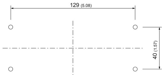
The bottom part of the housing is mounted with 4 screws (not in the scope of supply)
