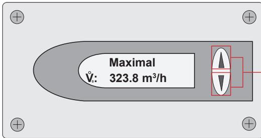
Press pushbutton UP and DOWN at the same time for >3s
