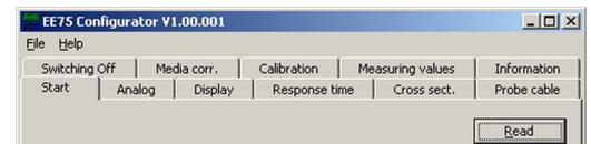
The "Start" tab is used to initiate communication with the connected transmitter.
