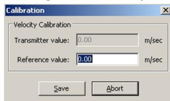
5. Enter the velocity displayed by the reference system in the "Reference value" input field.
