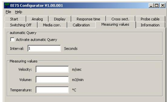
The configuration software allows the EE75 measuring values to be queried periodically on the "Measuring Values" index card.
