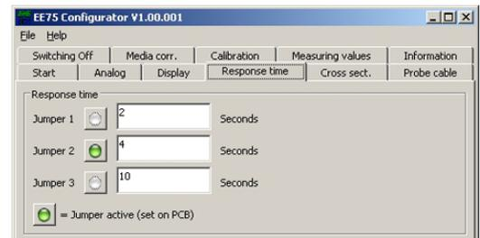
As described under Hardware, Section 5.2 - Jumpers for setting the velocity response time, three different response times can be set.
