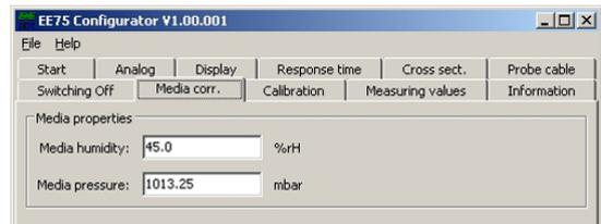
If e.g. the media pressure is significantly different, the actual values can be defined in the input field on the "Mediacorr." tab to obtain the best possible measuring results.
