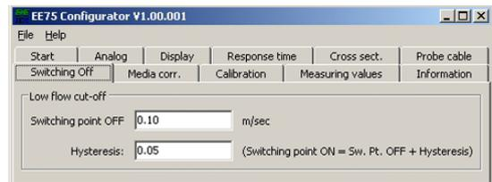
Switching point OFF and Hysteresis: (switching point OFF + hysteresis = switching point ON) can be defined in the input fields of the "Switching Off" tab.
