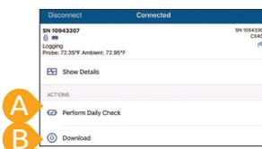
Tip: If you want to use InTempConnect in the future, download and stop the logger first and then log in as an InTempConnect User to reconfigure.
