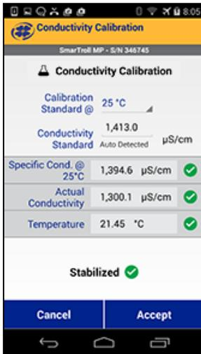
14. The calibration values are applied to the sensor and appear on screen. You can view a full calibration report for all sensors, or select **Done** to return to the Calibration Menu.
