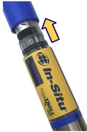
1. Remove the rubber bumper and blue top cap from the restrictor.
