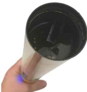
9. Move the solution in the calibration cell to ensure it has been in contact with the surface of the sensors and the inside of the calibration cell. If necessary, reinstall the blue top cap and gently shake.
