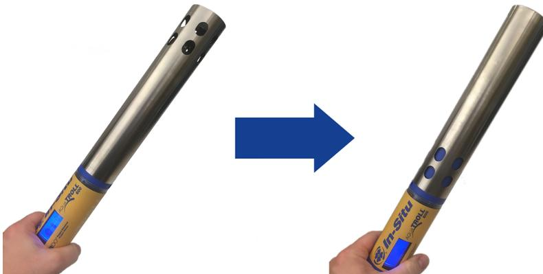
6. Invert the instrument so the sensors are facing up.
