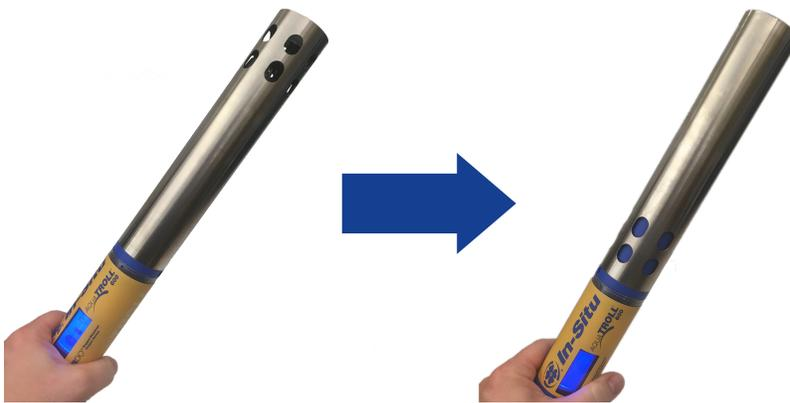
5. Invert the instrument so the sensors are facing up.
