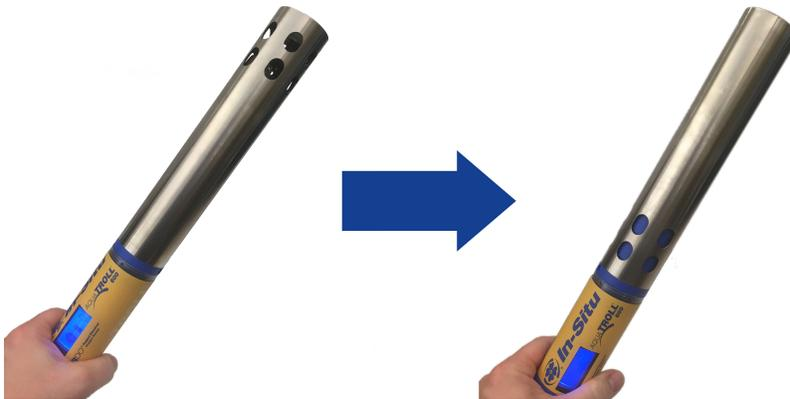
*Figure 8.1 Left: Deployment mode, Right: Calibration mode*
