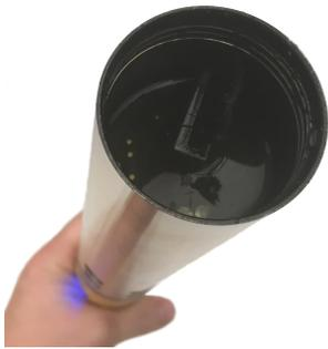
6. Move the solution in the calibration cell to ensure it has been in contact with the surface of the sensors and the inside of the calibration cell. If necessary, reinstall the blue top cap and gently shake.
