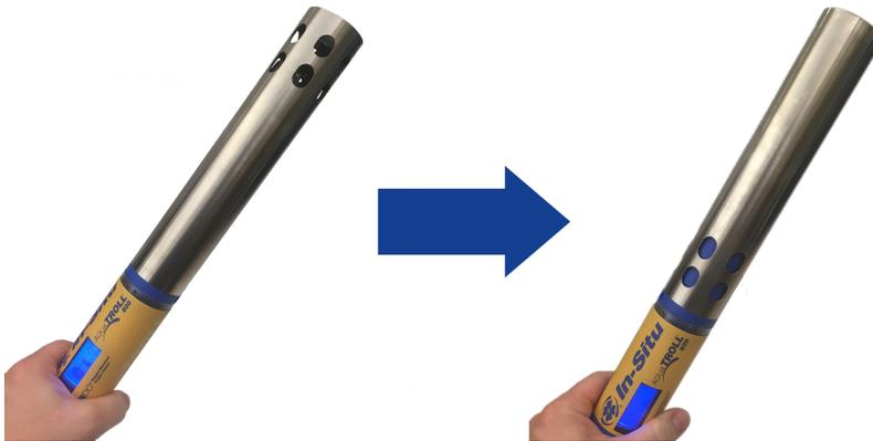
7. Invert the instrument so the sensors are facing up.
