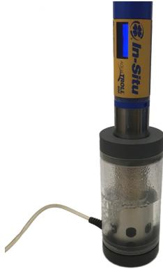
3. After the calibration chamber or bubbler have stabilized, perform the sensor calibration using VuSitu Mobile app or Win-Situ 5 software.
