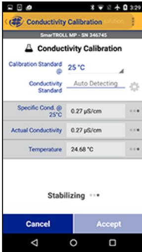
12. Check your bottle of calibration standard to determine the reference temperature. If necessary, tap the drop down list and select the appropriate reference temperature for the calibration.
