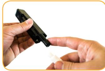
Apply a pea-sized drop of lubricant to sensor O-rings.
