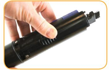
Insert pH/ORP sensor in empty sensor port.
