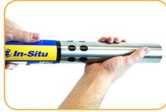
Replace restrictor with vent holes at base of instrument for calibration.
