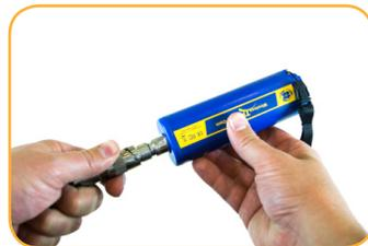
Align TROLL Com connector with cable end. Push and twist until you hear a click.
