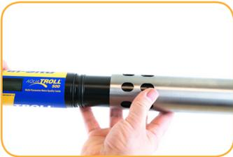
Remove the restrictor from the instrument.
