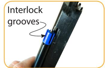
Sensor tongue must slide into blue motor interlock groove.
