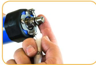
Ensure O-ring on instrument connector is clean.
