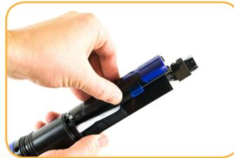
Insert RDO sensor in instrument sensor port.
