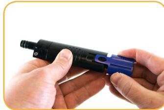
Install the RDO cap on the sensor.
