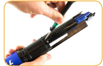
Lever the Allen wrench towards the top of the sonde to slide the sensor out.
