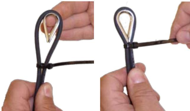
4. Place the second zip tie directly below the first and tighten.
