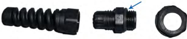
2. Twist the grommet through the drilled hole in the housing **with the O-ring against the outside of the housing**. Tighten the grommet to finger-tight, then turn it an additional half-turn with a 15-mm wrench.
