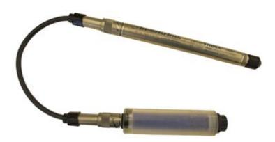
Extra large desiccant connected to RuggedCable System and Level TROLL Instrument
