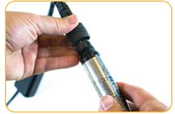
Connect cable to instrument and plug into PC's USB port.
