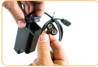
Open Rugged TROLL Com's battery compartment door. Insert 9-volt battery.
