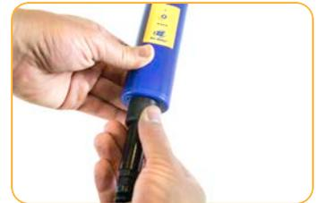
Connect cable to Wireless Rugged TROLL Com.
