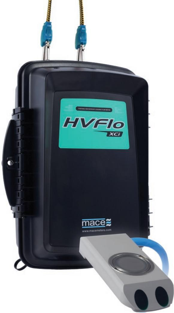
HVFlo Xci features MACE Doppler ultrasonic velocity sensors utilizing MACE Advanced Signal Processing (MASP) technology that “see” across the entire stream profile to give a true average velocity. MASP allows HVFlo Xci to produce superior results under a very wide range of hydraulic operating conditions.
