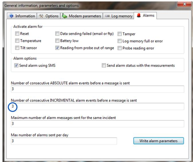
In Incremental Mode, alarms and warnings occur when the difference between two consecutive measurement values is less than the minimum threshold value or greater than the maximum threshold value. This difference means the alarm threshold is a slope instead of a fixed value.
