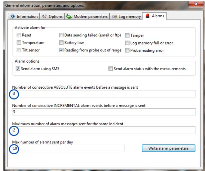
In Absolute Mode, alarms and warnings occur when a measurement value is less than the minimum threshold value or greater than the maximum threshold value.
