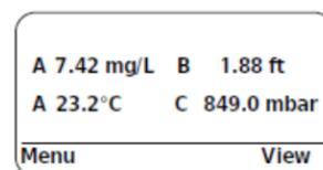
The Main Screen shows two parameters from Probe A, one parameter from Probe B and one parameter from the Con TROLL PRO. You can display four parameters at a time.
