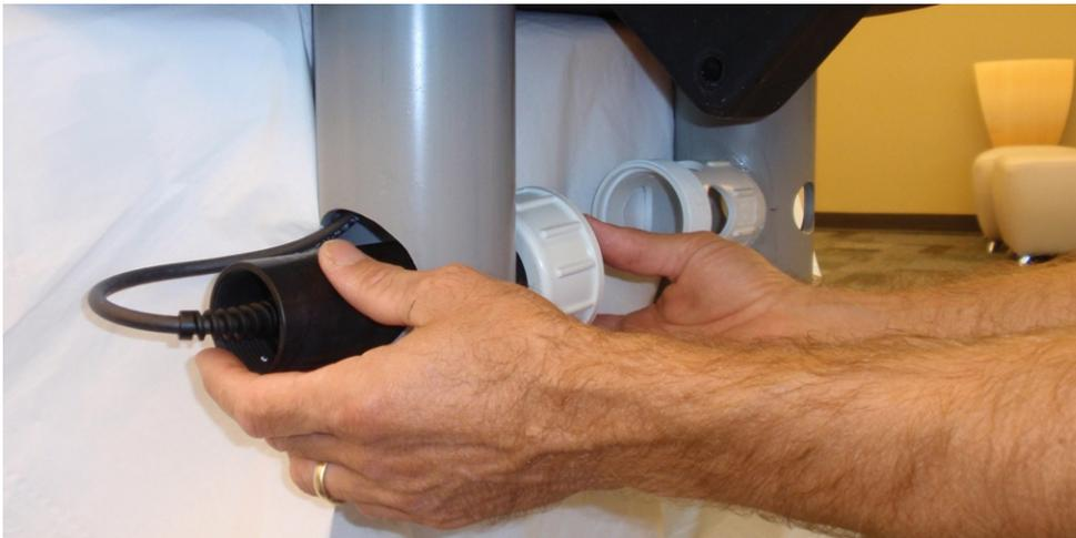
**Note:** Avoid allowing moisture, including atmospheric humidity, inside the cap. Keep the cap in its sealed packaging until you are ready to install it. Install promptly. Make sure that O-ring grooves are dry and the O-ring is not rolled or pinched inside the cap.
