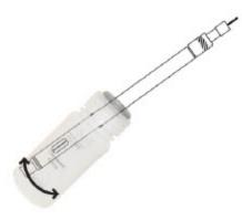
**TIP:** With the correct fill level, and the instrument held at a 45° angle, the air bubble in the Cal Cup will not intrude into the conductivity sensor.
