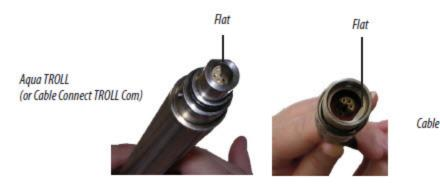
Note the pins on the instrument connector (one on each side) and the slots on the cable connector (one on each side).
