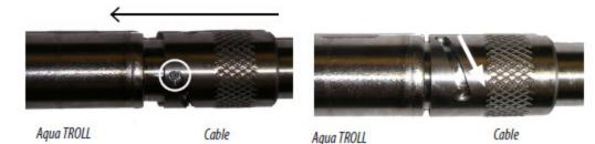
7. To attach a Cable Connect TROLL Com, first remove the desiccant from the cable by grasping the textured section of the cable connector in one hand and the desiccant in the other. Twist in opposite directions to unlock the desiccant from the cable.
